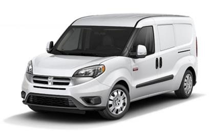
Isolated cargo space reduces odors and vapors from entering occupant compartment
